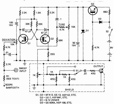
FIG. 1—MULTIVIBRATOR SIGNAL GENERATOR delivers sweep signal for i.f. circuit alignment.
