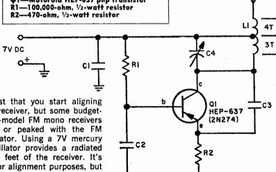
We don't suggest that you start aligning your stereo FM receiver, but some budgetpriced and early-model FM mono receivers can be aligned or peaked with the FM Alignment Oscillator. Using a 7V mercury battery, the oscillator provides a radiated signal within 10 feet of the receiver. It's strong enough for alignment purposes, but won't overload the front end.
