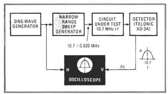
2. Performance second to none. Sine-wave generator output is approximately 0-2 V at frequencies below 100 Hz. Lower sweep rates produce a more stable scope pattern, because circuit response rings less. The detector may be any general peak-detecting type.
